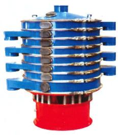
TEAHIVE-compact multideck Vibrograder ideally suited for final CTC tea grading. Heavy duty construction with specially designed vibro motor and springs ensures trouble free and consistent performance. Stainless steel meshes supplied with correct apertures end mesh diameter to ensure homogeneous sorting.
