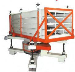
ROTOTEA is a Five Deck sorter with a rotary movement on a horizontal axis, fitted with different size of Stainless steel meshes. It sorts brokens and fannings.
