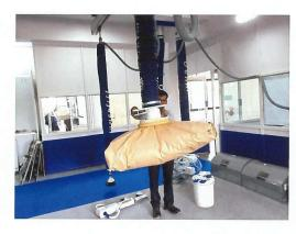
Vacuum bag lifter, which aims to facilitate the work of movement of the paper bags from the vibrator to the assembly of pallets. This work is currently carried out by operators, in case of using the rig tires would use only one operator for this operation & physical injury as a result of heavy lifting is avoided
