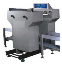
This is the vacuum packaging machine used in "tea industry" for packing CTC dust – up to 35 ~ 40 kgs. The powder can be filled into a 5 layer nylon co-extruded bag (vacuum bag) kept in a rectangular hopper (for giving shape). The filling can be performed using a semi automatic filling machine (Weigh metric). The vertical vacuum packaging machine performs evacuation, gas (upto 2 gases - if required ), sealing flushing operations.
