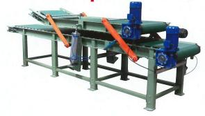
Specially designed for handling of Tea Filled Paper sacks. Paper sack will travel through the conveyors on Top and Bottom controlled by pneumatically operated Cylinders. The pressure air cylinders are provided at the sides for compression, the pressure will be applied to the Paper sack gradually while travelling and at the end of 5 meters travel, the Paper Sack will be flattened.
