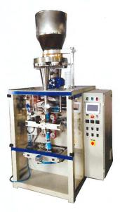
Fully automatic FFS Machine with PLC Control COLLAR TYPE, pneumatic bottom sealing with Pneumatic batch coding system, Pneumatic batch cutting with High speed telescopic adjustable SS Disc & Cup (Volumetric filling system to pack tea, Laminated Gusset Poly pouches in the following ranges:
