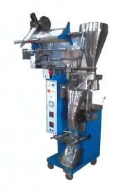
Automatic FFS Machine Clutch Break with PLC control Pneumatic sealing system, pneumatic batch coding with Adjustable Telescopic SS disc & cup to pack Tea dust 200 & 500 gms in laminated poly pouches
